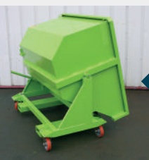
Stiffeners reinforce bin
