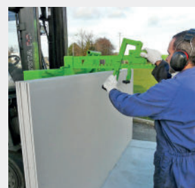
Easy loading by just sliding the boards to the right - After loading, the adjustment arms need to be repositioned to hold the remaining boards
