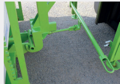
Handling trolley gripped by the spreader - Lever is unclipped by automatic locking of the hook onto the handling trolley with no intervention from the forklift driver
