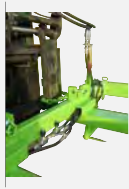
Hydraulic assembly with adjustment for telescopic arm
