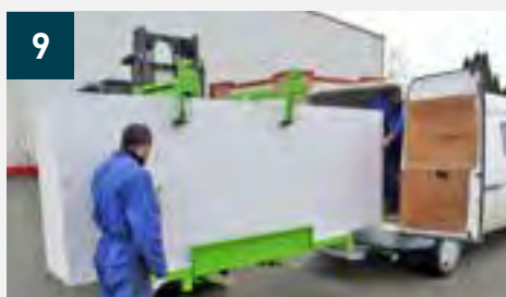
Easy loading by just sliding the boards to the right - After loading, the adjustment arms need to be repositioned to hold the remaining boards
