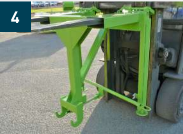
PK spreader put on forklift truck
