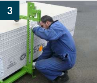
Adjustable retaining arms fitted
