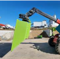
Dump position by tilting the forks
