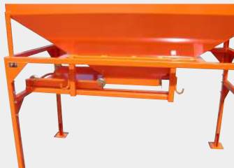
Sliding hatch on external rollers
