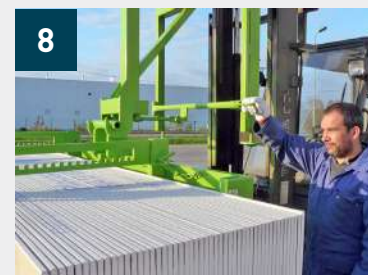
Lever clipped on to enable the spreader to be unhooked and removed
