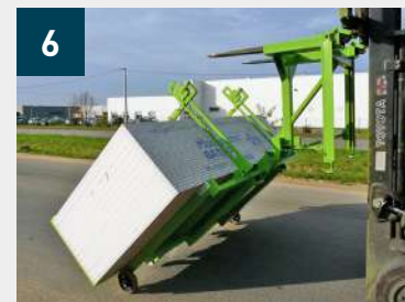
Trolley tilted vertically, the 4 high-density polyethylene feet prevent the ground from being marked
