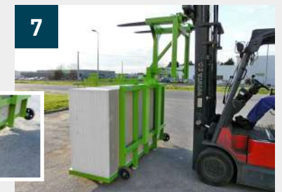
Trolley in unloading position before removal of the PK spreader
