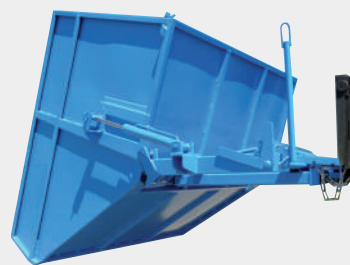
Deceleration cylinder for end of tipping process (VRP)
