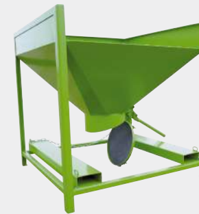
Round chute, sealed by eccentric lever
