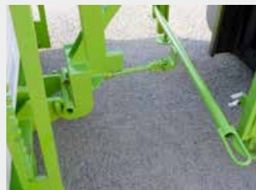
Handling trolley gripped by the spreader - Lever is unclipped by automatic locking of the hook onto the handling trolley with no intervention from the forklift driver
