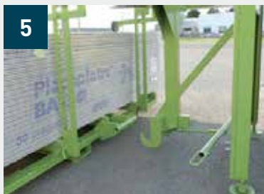
Handling trolley gripped by the spreader - Lever is unclipped by automatic locking of the hook onto the handling trolley with no intervention from the forklift driver
