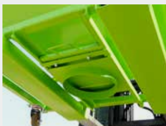
Basic sliding hatch for light products
