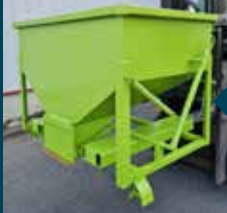
Controlled emptying achieved with the lever
