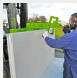
Easy loading by just sliding the boards to the right - After loading, the adjustment arms need to be repositioned to hold the remaining boards
