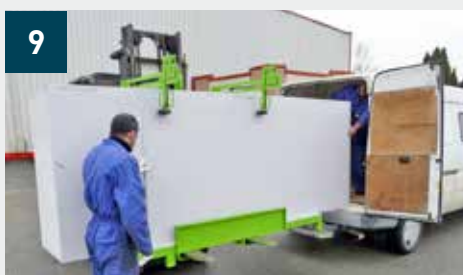
Easy loading by just sliding the boards to the right - After loading, the adjustment arms need to be repositioned to hold the remaining boards
