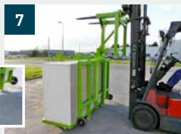
Trolley in unloading position before removal of the PK spreader
